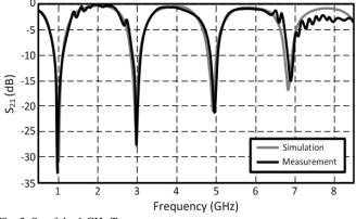
Fig. 3.  $S_{21}$  of the 1 GHz T-resonator.
