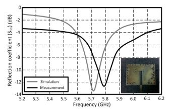
Fig. 13. Simulated and measured reflection coefficient  $(S_{11})$  of the inkjet-printed SIW cavity resonator.
