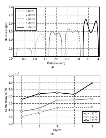
Fig. 1. Thickness and conductivity of inkjet-printed traces: (a) thickness (b) conductivity.
