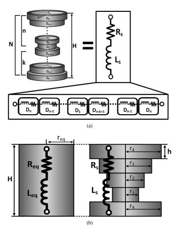
Fig. 10. (a) Equivalent circuit model of a stepped via and (b) equivalent via model of a cylindrical via and a stepped via.
