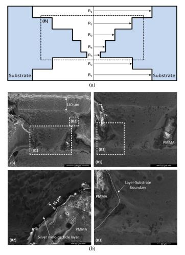
Fig. 8. (a) Geometry of stepped via hole and (b) SEM images of metalized stepped via hole: side view
