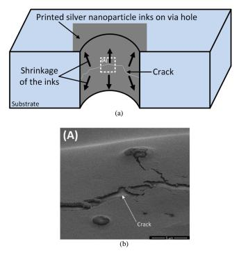
Fig. 5. (a) Crack formation of inkjet-printed silver nanoparticle on a straight vertical via hole and (b) SEM image of the crack on the metalized via hole.
