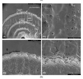
Fig. 7. (a) Geometry of stepped via hole and (b) SEM images of metalized stepped via hole: top view  $% \left( \frac{1}{2} \right) = 0$
