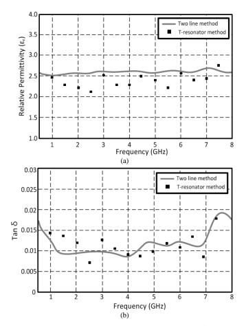
Fig. 4. Extracted (a) relative permittivity ( $\varepsilon_r$ ) (b) loss tangent (tan  $\delta$ )
