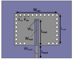
Fig. 12. Geometry of the SIW cavity resonator:  $W_{feed} = 2.5 \text{ mm}$ ,  $L_{feed} = 10 \text{ mm}$ ,  $W_{cav} = 32 \text{ mm}$ ,  $L_{cav} = 22.4 \text{ mm}$ ,  $D_{via} = 1.6 \text{ mm}$ ,  $P_{via} = 3.2 \text{ mm}$ ,  $L_{mat} = 17 \text{ mm}$ ,  $W_{mat} = 0.6 \text{ mm}$  and  $W_{in} = 1.25 \text{ mm}$ .
