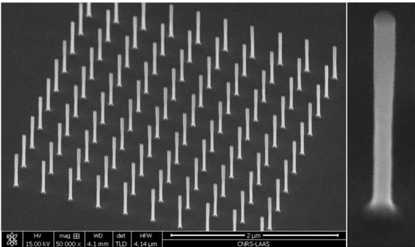
Figure 4. GaAs nanowires array (diameter = 40nm).
