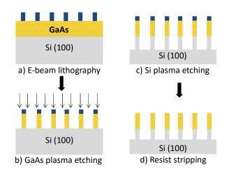
Figure 1. Process flow chart: a) First step is electron beam lithography with a negative resist (HSQ). b) ICP-RIE of GaAs thin layer by stopping on silicon substrate. c) ICP-RIE of silicon substrate. d) Last step is a wet etching to remove inorganic resist.
