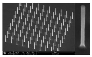
Figure 4. GaAs nanowires array (diameter = 40nm).
