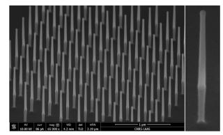
Figure 5. Heterostructured GaAs-Si nanowires array (diameter = 40nm) on Si(100) substrate.
