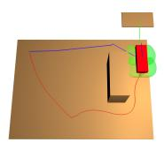
Fig. 6: The goal of this problem is located on the platform. While the blue trajectory is the shortest to reach to the shown position for a simplified robot, only the red one allows to reach the velocity required to perform the upcoming jump in green. Local methods won't be able to escape the blue trajectory, contrary to our planner.
