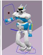
Fig. 3: Approximation of contact locations in  $\mathcal{P}_1$ . Left: the blue polygons represent the intersection between the reachable workspace and the environment. The centroid of this intersection serves as the estimated center of the contact location (black sphere), from which the contact extremities are extrapolated (red sphere). Right: the actual contact locations generated during  $\mathcal{P}_2$ .
