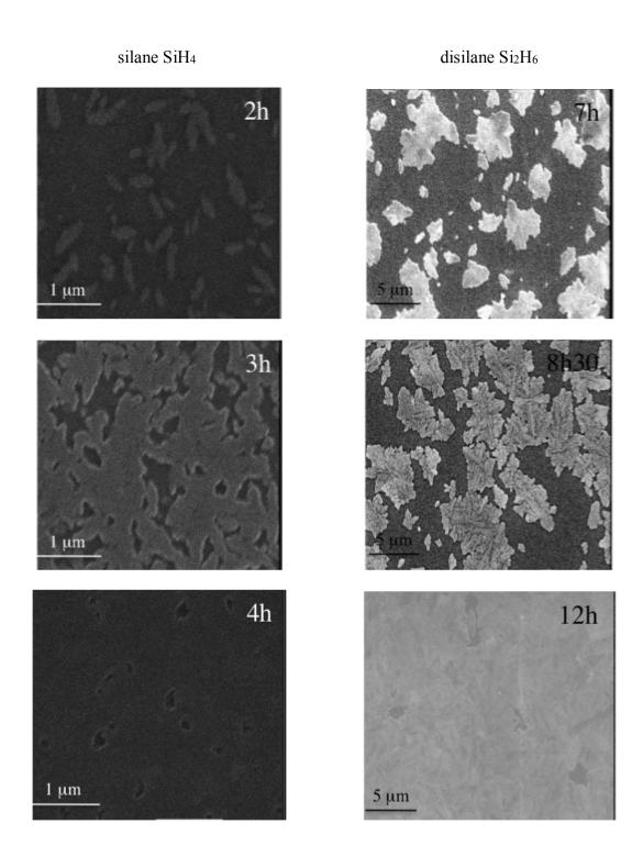
Figure 4: Microstructures of silicon films for different annealing durations at  $600^{\circ}$ C for the silane SiH4 and disilane Si<sub>2</sub>H<sub>6</sub> gaseous sources
