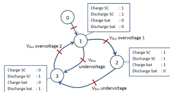
Fig. 6. State diagram of the OPA MG
