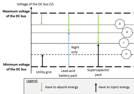
Fig. 9. Principle of LVDC OPA MG energy management
