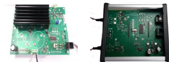
Fig. 5. Power electronics developed in the LAAS On the left - 1kW bidirectional DC/DC converter, On the right – Power converter control board.
