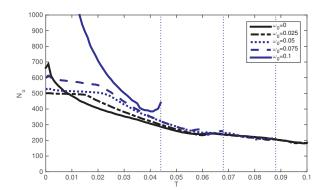
Fig. 2. Evolution of the average number of control updates  $N_u$  with respect to the dwell time parameter T for several values of  $\omega_0$ . The vertical dotted lines represent the limit values of the dwell time parameter for which the conditions of Theorem 3 are feasible for  $\omega_0 = 0.1$  (left),  $\omega_0 = 0.075$  (middle) and  $\omega_0 = 0.05$  (right).
