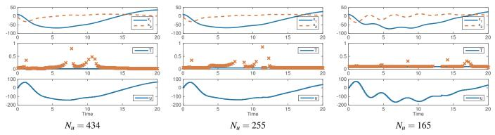
Fig. 1. Figure representing the state of the plant  $x_p$ , the inter-sampling times (with the dwell time T) and the control input u issued from Theorem 2 with T = 0.02 (left), T = 0.05 (middle) and T = 0.10 (right).
