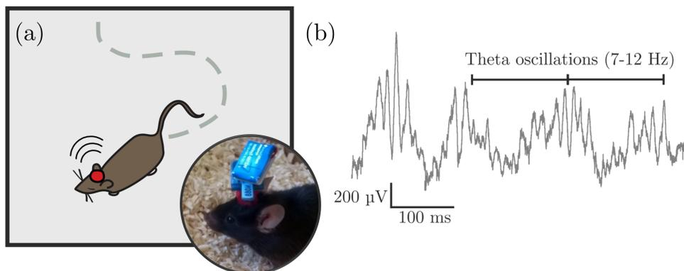
Figure 3: **(a)** Schematic representation and photograph of an *in vivo* wireless recording session. A freely-moving mouse is actively exploring an unknown environment, and its hippocampal activity is recorded wirelessly with a Parylene-based neural probe connected to a commercial headstage and battery (in blue). **(b)** Typical hippocampal activity displayed during a recording session. Spatial navigation of the animal induces large Theta oscillations at around 7-12 Hz.
