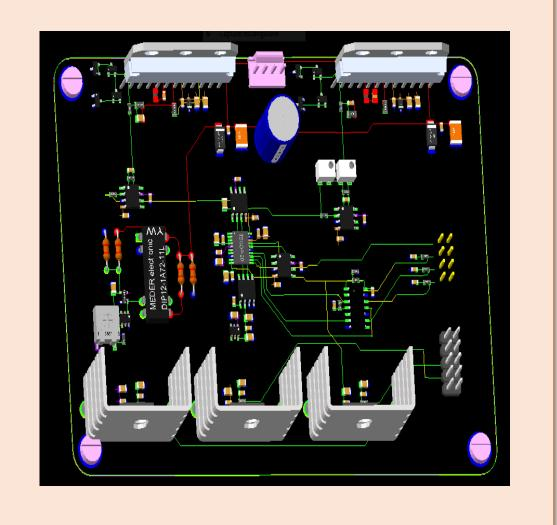
memade electronic board to drive the fast 2 actuator, consists of a 20-bit DAC and two (100V, 500 kHz) amplifiers to drive the two opposite ceramic piezos. The 20-bit word is generated by NI-9401 digital ouput module via SPI bus at 40MHz.
