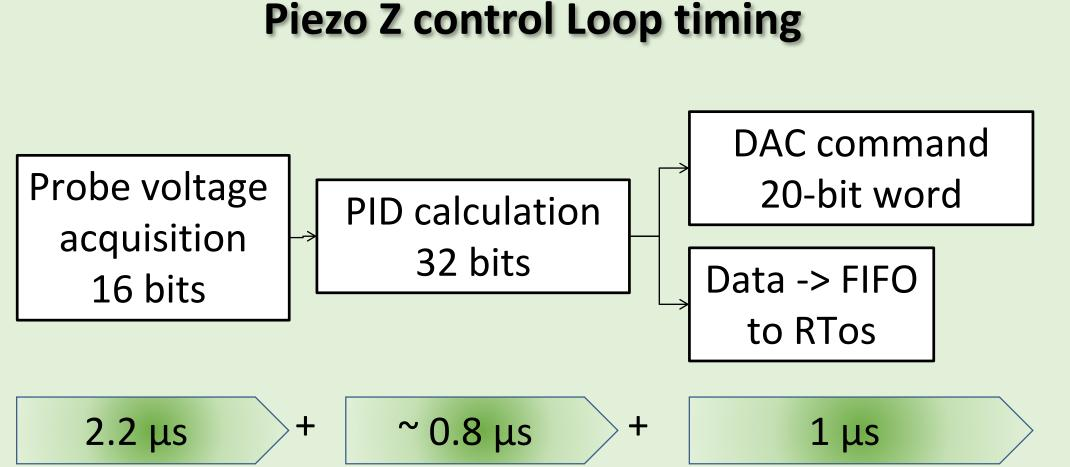
FPGA: microscope Z feedback operations take about 4 μs to complete. It executes every 1 µs with pipelining method.
