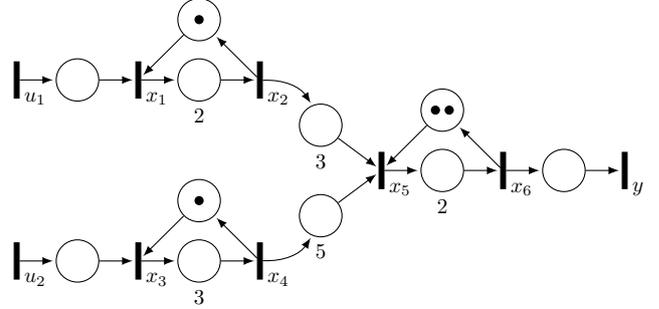
Figure 2: A TEG of an automated assembly line.
