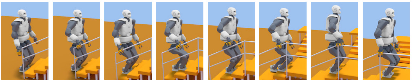
(c) Snapshots of the climbing 15-cm high steps motion with stair railing by the TALOS robot in simulation.
