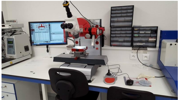
Figure 14 – Machine de shear et pull tests Xyztec Condor Sigma
