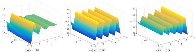
Fig. 2: Chart of u for system (30) with the parameters:  $u_0(x) = (\cos(\pi x) + 1) \frac{KX_0}{2}$ ,  $X_0 = \begin{bmatrix} 1 & 1 \end{bmatrix}^\top$ ,  $v_0(x) = 0$  and  $c_0 = 0.15$  for 3 values of c. These results are obtained using Euler forward as a numerical scheme.
