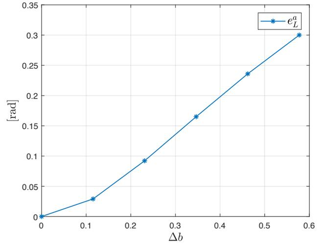
Fig. 8: Load position and attitude errors when the load mass known by the controller differs from the real one.
