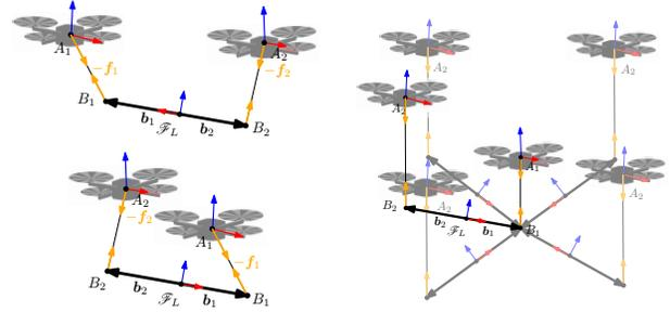
(a) Two equilibria for  $t_L \neq 0$ . On the top and on the bottom one equilibrium configuration in  $\mathcal{Q}^+(t_L, \bar{q}_L)$  and  $\mathcal{Q}^-(t_L, \bar{q}_L)$ , respectively. (b) Five of the possible infinite equilibria in  $\mathcal{Q}(0, \bar{q}_L)$ . In vivid color the configuration  $\bar{q}$ . The final load pose depends on the initial conditions.
