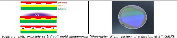
Figure 1. Left: principle of UV soft mold nanoimprint lithography. Right: picture of a fabricated 2'' GMRF sample.
