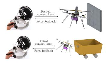
Fig. 5: The scenarios of aerial teleoperation for physical interaction with contact considered in [28]. Top: docking to a surface. Bottom: pushing a cart.
