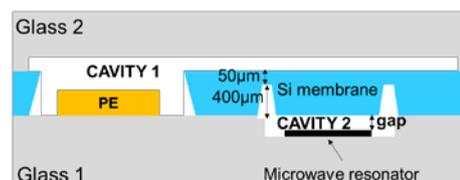
Figure 1. Cross section of the nuclear radiation sensor.
