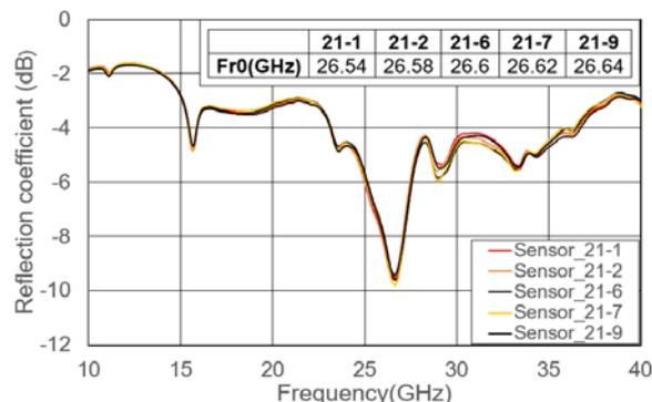
Figure 3. Measured reflection coefficient vs frequency at the input port of 5 nuclear radiation sensors (called here 21-1, 21-2, 21-6, 21-7 and 21-9) before nuclear irradiation.
