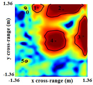
Figure 15. 2D display of the nuclear radiation sensor in a cut-plane at  $z=7.50\text{m}$ . A contour analysis is performed for an initial level of  $-40\text{dB}$ . The contour No 4 corresponds to the nuclear radiation sensor echo.
