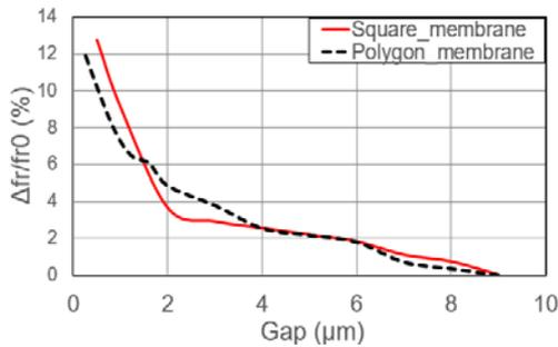
Figure 5. Frequency shift depending of membrane position for two membrane geometries: square and polygon (octagonal) membranes.
