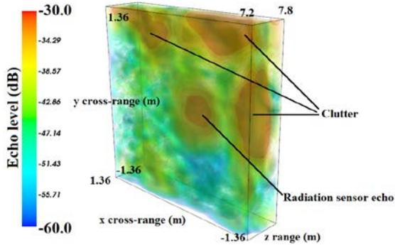
Figure 14. 3D echo level display of the nuclear radiation sensor. The radiation sensor echo is surrounded by undesirable echoes (clutters).
