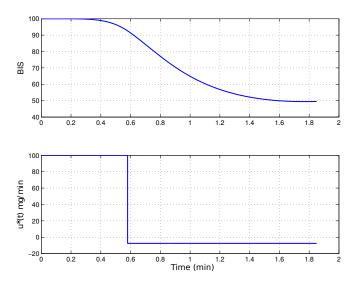
Fig. 6. The BIS evolution in response to the minimum time control  $u^*(t)$  which consists at keeping u(t) at its maximum  $U_{max} = 100mg/min$  for about 0.55 minutes then switch to its minimum  $U_{min} = -u_e$  for 1.3 minutes.
