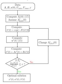
Fig. 3. Flowchart for the computation of the optimal control solution to Problem (5)
