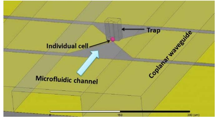
Fig. 1. Schematic view of the microwave biosensor, which includes a 5  $\mu\text{m}$  capacitive gap in coplanar waveguide with a microfluidic channel placed on top; the cell is blocked due to a mechanical trap.
