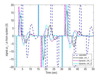
Figure 10 – roll solicitation of +40 deg at time t = 1 s followed by a step of -60 deg at time t = 15 s and a step of +60 deg at time t = 30 s: comparison of the signal  $\dot{x}_a$  used in Equation (3) for the saturated (no compensation of the saturation) and designed static and anti-windup cases
