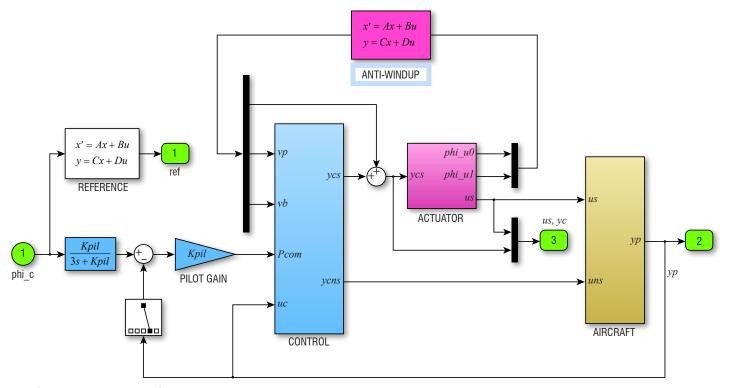
Figure 3 – Nonlinear closed-loop Simulink implementation of anti-windup AW, for lateral aircraft simulations
