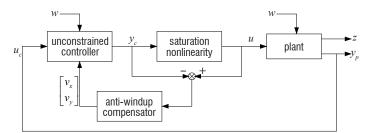
Figure 1 – Anti-windup principle
