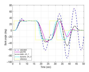
Figure 12 – roll solicitation with a 3211 type input of amplitude  $\pm$  30 deg with a  $\Delta t = 5$  s: comparison between the performance outputs for the saturated (no compensation of the saturation), standard anti-PIO and designed static and anti-windup cases
