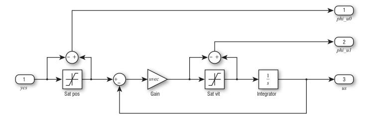
Figure 4 – Detailed view of the magnitude and rate limitation system
