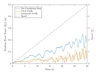
Fig. 6: Position error norm  $\|E_p\|$  when ramping the speed on the circle trajectory from  $0\,\mathrm{m\,s^{-1}}$  up to  $5\,\mathrm{m\,s^{-1}}$  in  $30\,\mathrm{s}$  without considering rotor drag (solid blue), with drag coefficients estimated on the circle trajectory (solid red), and with drag coefficients estimated on the lemniscate trajectory (solid yellow). The reference speed on the trajectory is shown in dashed purple.
