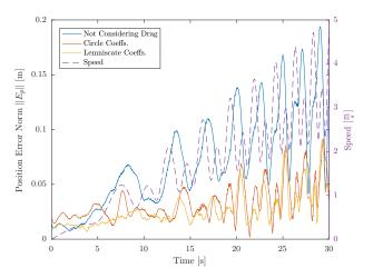
Fig. 7: Position error norm  $\|E_p\|$  when ramping the maximum speed on the lemniscate trajectory from  $0\,\mathrm{m\,s^{-1}}$  up to  $5\,\mathrm{m\,s^{-1}}$  in  $30\,\mathrm{s}$  without considering rotor drag (solid blue), with drag coefficients estimated on the circle trajectory (solid red), and with drag coefficients estimated on the lemniscate trajectory (solid yellow). The reference speed on the trajectory is shown in dashed purple.
