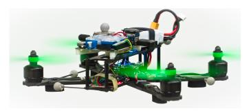
Fig. 1: First-person-view racing inspired quadrotor platform used for the presented experiments.
