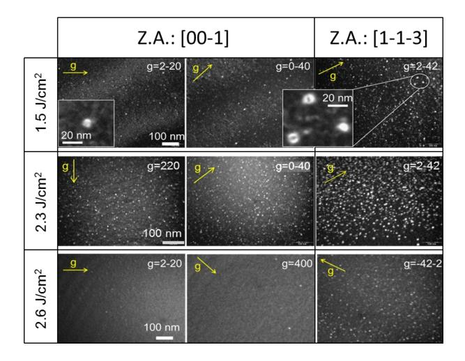
**Figure 2.** Plan-view WBDF TEM images of B implanted samples annealed by *(top row)* 10 pulses at 1.5 J/cm<sup>2</sup> (non-melt), *(middle row)* 1 pulse at 2.3 J/cm<sup>2</sup> (partial melt above the  $R_p$ ), *(bottom raw)* 1 pulse at 2.6 J/cm<sup>2</sup> (partial melt beyond the  $R_p$ ). Images are taken using different zone axes and diffracting vectors. *Left column*: Z.A.: [00-1], g=<220>; *Middle column*: Z.A.: [00-1], g=<400>; *Right column*: Z.A.: [1-1-3], g=<422>.
