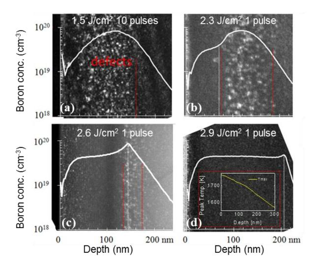
**Figure 1.** SIMS boron profiles and corresponding cross-section TEM images from B implanted samples annealed by *(a)* 10 pulses at  $1.5 \text{ J/cm}^2$  (non-melt), *(b)* 1 pulse at  $2.3 \text{ J/cm}^2$  (partial melt above the  $R_p$ ), *(c)* 1 pulse at  $2.6 \text{ J/cm}^2$  (partial melt beyond the  $R_p$ ) and *(d)* 1 pulse at  $2.9 \text{ J/cm}^2$  (full melt). *Inset:* Calculated depth variation of the peak temperature reached during laser annealing at  $2.6 \text{ J/cm}^{-2}$ .
