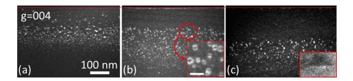
**Figure 5.** Cross section WBDF TEM images (surfaces are indicated by the red dashed line) of the Silicon implanted sample annealed by (a) 10 pulses at 1.5 J/cm<sup>2</sup> (non-melt), (b) 1 pulse at 2.6 J/cm<sup>2</sup> (partial melt above  $R_p$ ). Scale bar in the inset is 20 nm, (c) 1 pulse at 2.9 J/cm<sup>2</sup> (partial melt below  $R_p$ ). Inset: HREM image of a loop with (001) habit plane.
