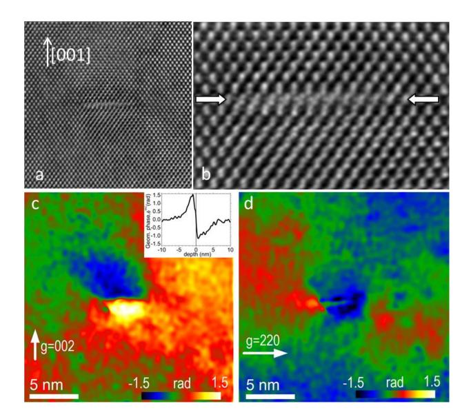
**Figure 3.** Geometric phase analysis of a dislocation loop in a B implanted sample annealed by 1 pulse at 2.6J/cm<sup>2</sup>. (a) HRTEM image in [-110] orientation; (b) enlarged view of the dislocation. The habit plane is (001); (c) geometric phase image of the 002 lattice fringes; (d) geometric phase image of the 220 lattice fringes.
