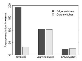
Fig. 7. Average resolve time on switch failure.
