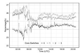
Fig. 4. Load Balancing real world performance.
