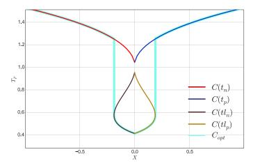
Fig. 9. Shortcut trajectories introduces discontinuities in the time-optimal curve  $\mathcal{C}_{opt}$ .  $(J_{min}=-40,J_{max}=40,A_{min}=-30,A_{max}=30,V_{min}=-30,V_{max}=30,a_i=20;v_i=-4.99;a_f=20;v_f=4.99)$ .
