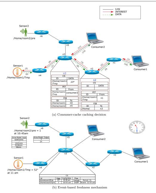
FIGURE 2. An example with the NDN architecture using consumer-cache caching strategy and event-based freshness mechanism
