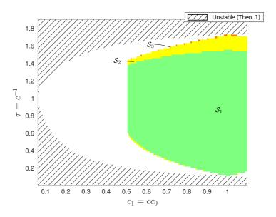
Figure 5: Stability areas for system (1) with matrices defined in (42) and  $c_1 = cc_0$  and  $\tau = c^{-1}$  obtained using CTCR and Theorem 4. The hatched area is the exact unstable area, the remaining area is the exact stable area as detected by CTCR. The colored areas are stated as stable for Theorem 4 at an order N = 3. The color scale represents the stability area depending on the order N considered. The areas marked as  $S_i$ is the stable area up to an order *i*.
