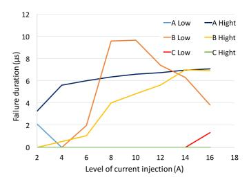
Fig. 7. Failure duration depending on current injection for a pulse wide of 300ns.
