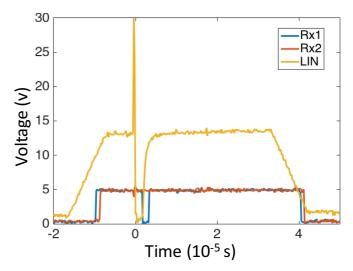
Fig. 10. LIN A master, LIN C slave, TLP generator set with 16A TLP with 300ns pulse wide.
