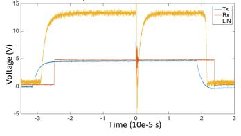
Fig. 4. LIN C with a perturbation at times 0, the TLP generator is set with 8A for 300ns pulse wide
