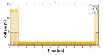
Fig. 11. LIN C master, LIN B slave, TLP generator set with 10A TLP with 300ns pulse wide. LIN communication lost during 9.4ms
