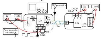
Fig. 8. Schematic of the test bench for LIN network characterization
