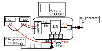
Fig. 3. Schematic of the test bench to charaterize one LIN
