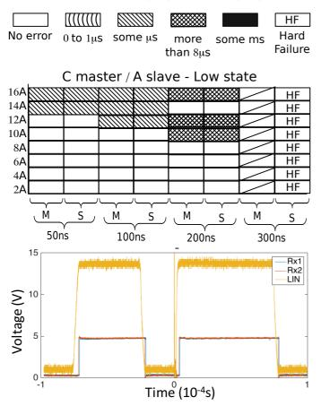
Fig. 9. LIN C master, LIN A slave, TLP generator set with 10A TLP with 200ns pulse wide. ESD event (time 0) durring a LIN low state, stuck the LIN bus in hight state.
