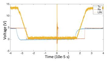
Fig. 6. LIN A with a perturbation at times 0, the TLP generator is set with 2A for 200ns pulse wide
