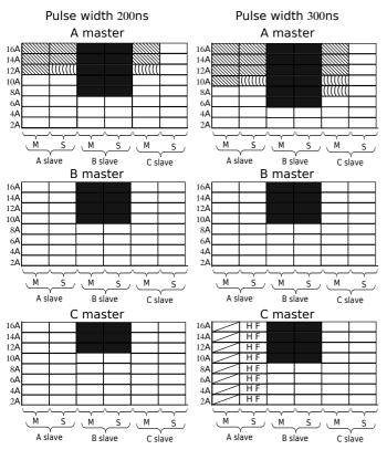
How to read these tables: Each colon represents the failure observed following the severity reported in table II. As an example, graph on left top reports the failures while component A is in master mode. The pair of colons (M & S) reports the configuration where A, B, and C are in slave mode respectively from left to right. Colon on reports the failure on master and colon two on the salve.
