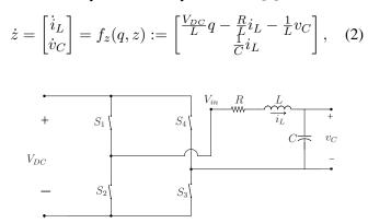
Fig. 1: Single-phase DC/AC inverter circuit diagram.
