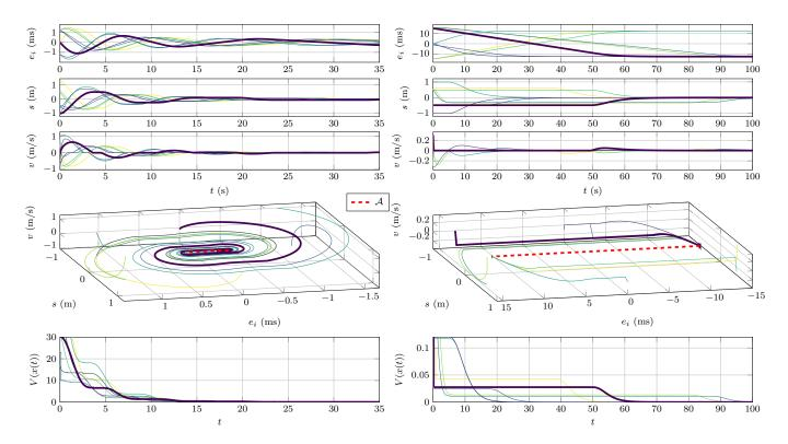
Fig. 2. Top: solutions to (4) for different initial conditions. Center: phase portraits for the same solutions. Bottom: Lyapunov-like function V in (13) evaluated along the same solutions. The left (resp., right) column corresponds to  $(k_v, k_p, k_i) = (6.4, 3, 4)$  (resp., (1.5, 0.66, 0.08)), and both share  $f_c = 1$  m/s<sup>2</sup>.
