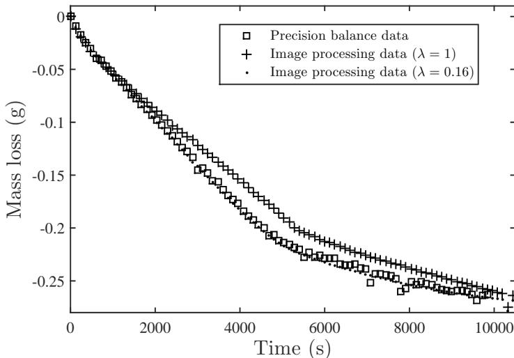
FIGURE 5. Mass loss during evaporation of heptane in a large micromodel ( $h = 525 \mu\text{m}$ ). Squares: data from a precision balance; crosses, respectively dots: data from liquid volume measurements by image processing with  $\lambda = 1$  (no liquid in the meniscus region), respectively  $\lambda = 0.16$ .
