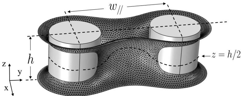
FIGURE 4. a) Typical liquid bridge capillary shape obtained from Surface Evolver. The liquid bridge is trapped between two cylinders and confined between two flat surfaces located in the  $z = 0$  and  $z = h$  planes (not displayed). The two cylinders, of diameter  $d_c$  appear in light gray and are separated by  $w_{//}$  (here,  $w_{//} = d_c$ ). The contact angle between the liquid and the solid surfaces is  $0^\circ$ .
