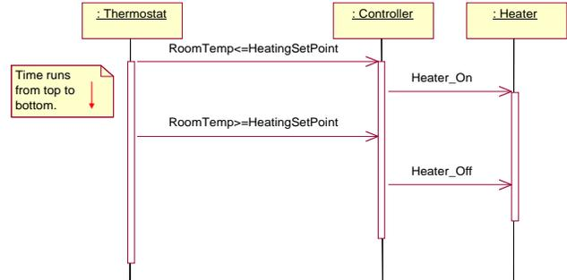
Figure 8. Sequence diagram for building heating mode.
