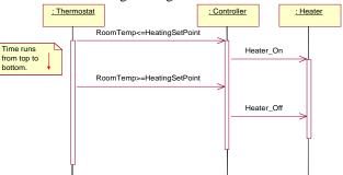
Figure 8. Sequence diagram for building heating mode.
