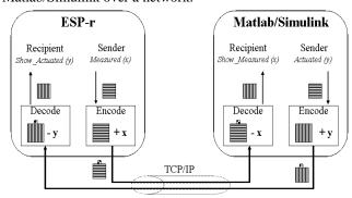
Figure 5. A distributed dynamic mechanism for building control and performance simulation.
