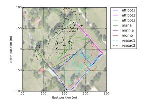
Fig. 5: Trajectory performed by the robots during the mission with only delays (no online repair needed). *ressacs* are aerial robots as shown in Fig. 1, *effibots* are ground robots that can evolve on paved roads, other robots are all-terrain ground robots as shown in Fig. 1.
