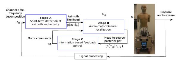
Fig. 1: The three-stage framework to active binaural localization. This paper addresses Stage C.
