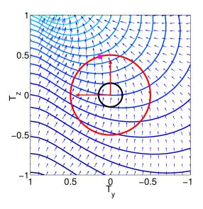
Fig. 5: Contour lines and local gradient vectors of the criterion  $F_k(T_y, T_z, 0)$  w.r.t. the translation variables  $T_y, T_z$ , *i.e.*, when no subsequent rotation is applied to the head ( $\phi = \phi_0 = 0$ ). The red circle delimits the admissible translations. The magenta spot depicts the constrained local maximum.
