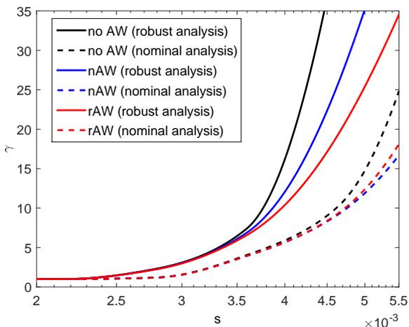
Fig. 2.  $\mathcal{L}_2$  gain estimates for the nonlinear closed-loop systems with and without anti-windup compensator. Both robust (solid) and nominal (dashed) analysis are considered to assess the performance of robust (blue,  $D_{aw}^{rand}$ ) and nominal (red,  $D_{aw}^{nom}$ ) compensators with respect to the system without anti-windup augmentation (black).
