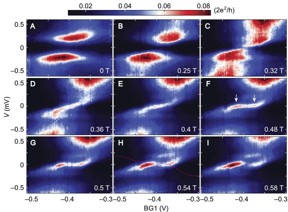
**Fig. 2. The emergence of the ZBP.** (A to I) Conductance maps in bias voltage  $V$  versus  $BG1$  at different magnetic fields indicated in the lower right corner of each panel. The arrows in (F) mark the ZBP onset gate voltages plotted in Fig. 3. The dashed line in (H) is obtained by tracing the visible maximum in subgap conductance and flipping the resulting trace around  $V = 0$  mV.
