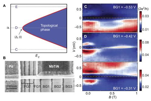
**Fig. 1. ZBP in a nanowire device controlled by gate voltages.** (A) Topological phase diagram described by Eq. 1. Dashed lines indicate settings of  $\mu$  in (E), (D), and (C). (B) Scanning electron micrograph of the device used in this work. An InSb nanowire is half-covered by a superconductor NbTiN and normal metal Pd contact. The nanowire is placed on FG and BG metal gates. (C to E) Differential conductance maps in bias voltage V versus magnetic field B at three different settings of BG1.
