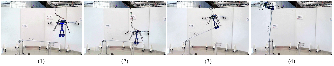
Fig. 6: Time-lapse of the OTHex in the bar lifting experiment, from left to right; (1) contact free-flight, (2) grasping the horizontal bar, (3) lifting the bar, (4) bar just lifted, inverting the motion.
