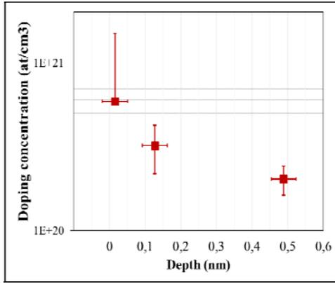
**Fig. 1:** Depth distribution of the active dopant concentration as determined by Differential Hall effect measurements from the SiGeOI sample implanted with Boron and laser annealed at an energy density of  $0.68 \text{ J/cm}^2$ .
