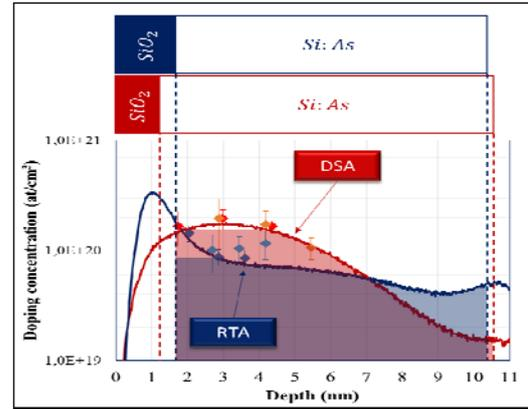
**Fig. 2:** Depth distribution of active dopant concentration for DSA and RTA processes measured by DHE (colored dots) compared to their respective SIMS (colored lines) from the 11 nm SOI samples implanted with arsenic at the same dose ( $10^{14} \text{ at/cm}^2$ ). Colored areas in the graph correspond to the active dose. Diagrams above graph zone represent the layers dimensions measured by ellipsometry.
