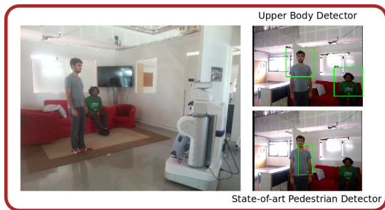
Figure 1: Output of our proposed detector (top right) and state-of-art pedestrian detector (Dollár et al., 2014), bottom right, in an HRI context.
