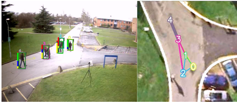
Fig. 6 Social forces representation. In the left image, we depict the output of our framework with IMM-PF SF. The four trackers are projected to the world plane through camera calibration (right image). The (directed) edges connect the trackers which interact with each other. Edges of same color correspond to the same tracker.
