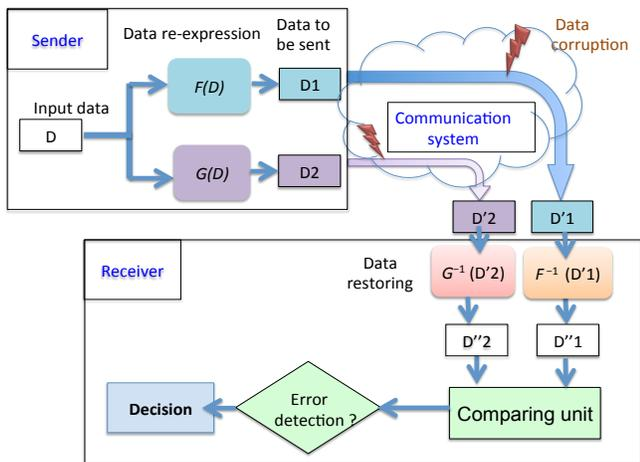
Fig. 8. Overview of Data diversity approach for communication integrity
