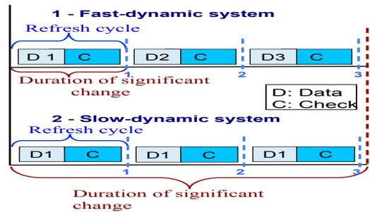
Fig. 3. Comparison between fast-dynamic and slow-dynamic properties
