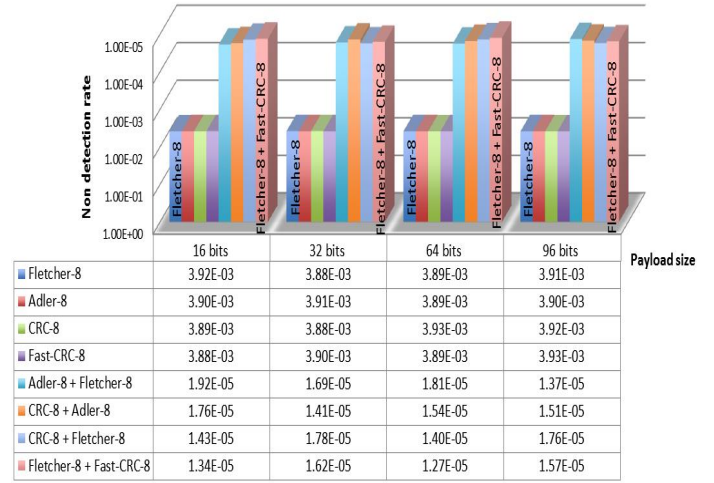
Fig. 5. The non detection rates of different error detection policies based on single or multiple 8 bits error detection bits
