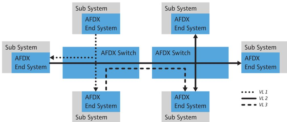
Figure 5: Virtual Link topology. Source: AFDX White paper [16]
