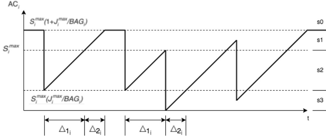
Figure 16: Frame-based policing parametrization to model as TPN
