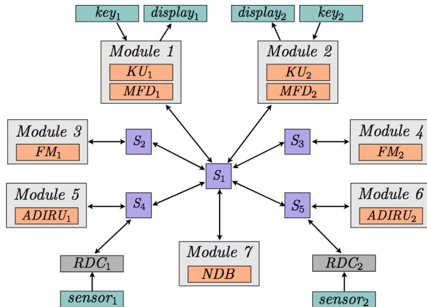
Figure 10: Flight Management System network architecture. Source: Lauer [9]
