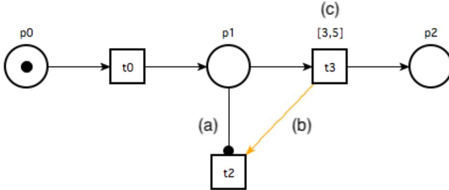
Figure 2: Petri net with mentioned extensions: (a) tokens from  $p_1$  will not be removed when firing transition  $t_2$ ; (b) transition  $t_2$  cannot be fired if  $t_3$  is enabled ( $t_3$  has higher priority over  $t_2$ ); (c) transition  $t_3$  can only be fired within the time interval  $[3, 5]$  time units after it became enabled.
