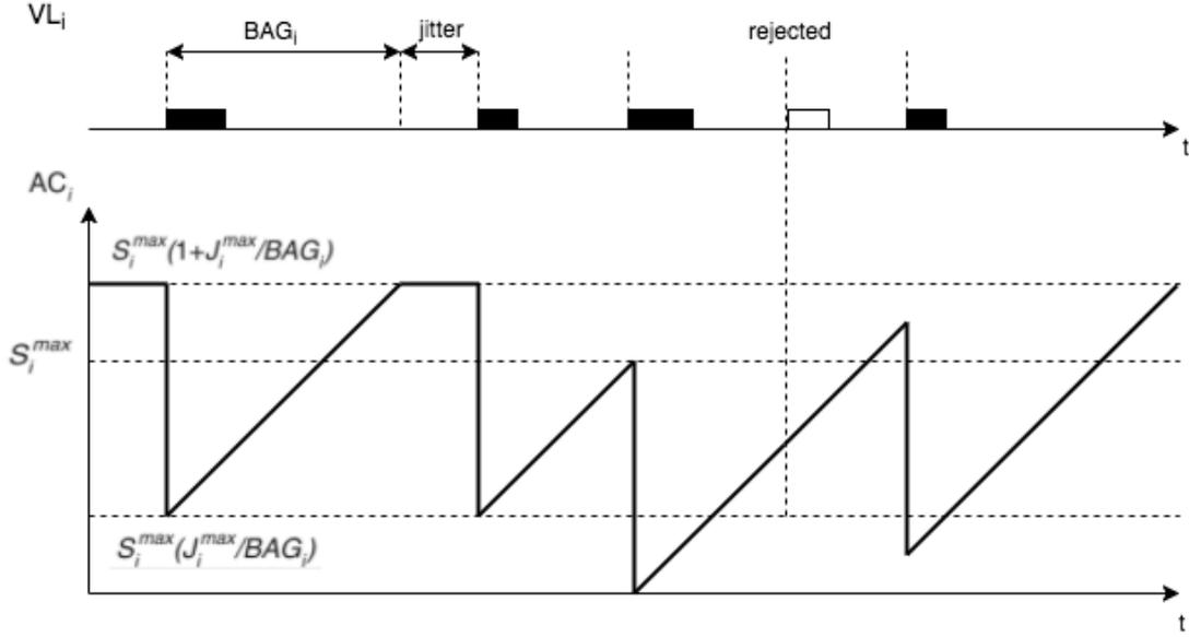
Figure 15: Example of frame-based traffic policing
