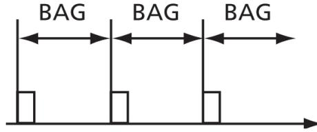
Figure 7: Bandwidth Allocation Gap. Source: Developing AFDX Solutions [1]
