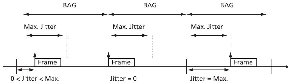
Figure 8: Jitter Defined. Source: Developing AFDX Solutions [1]
