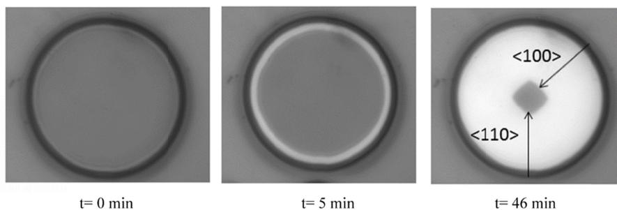
Fig. 1. In situ top images of laterally oxidized circular mesas during the oxidation process at three different process times. The mesa diameter is 60 $\mu\text{m}$ , and the oxidized zones appear in white.
