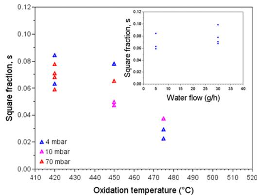
Fig. 4. Square fraction (anisotropy) of the oxide aperture (diameter around 6 $\mu$ m) obtained from a 35- $\mu$ m-diameter Al<sub>0.98</sub>Ga<sub>0.02</sub>As circular mesa versus process temperature, and (inset) versus water flow for a process temperature of 420°C.
