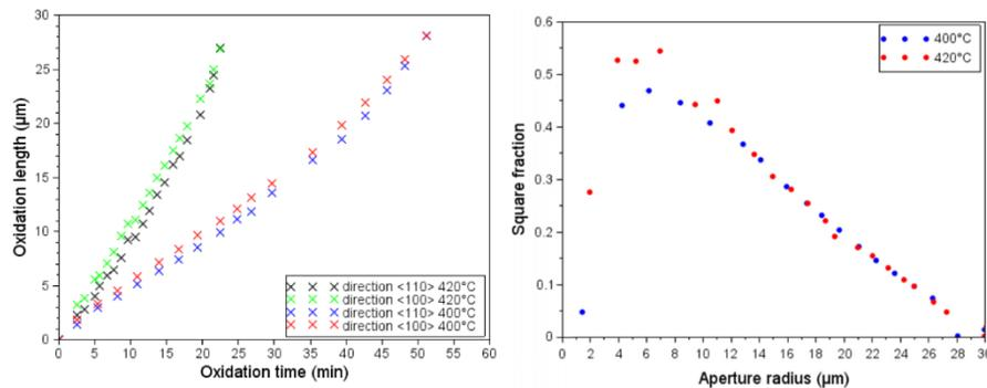
Fig. 2. left: Evolution during the process time of the oxidation depth along the  $\langle 110 \rangle$  and  $\langle 100 \rangle$  crystallographic directions for oxidations of a 70-nm-thick AlAs layer carried out from 30 $\mu\text{m}$ -radius mesa at a temperature of 400 and 420°C, a pressure of 500 mbar and a water flow of 5 g/h, and, right, associated anisotropy analysis in terms of square fraction.
