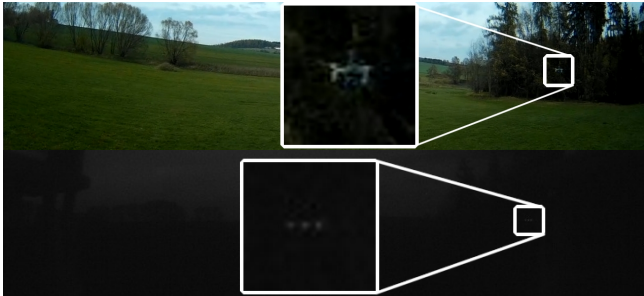
Fig. 3: An extreme case of long range and hard to separate background. In the visible spectrum the UAV is difficult to locate even by the human eye and today's popular CNN methods [7], while in UV the three markers are clearly visible as unique peaks in brightness and can easily be detected by the proposed system.
