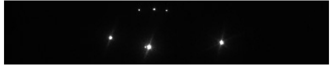
Fig. 6: Relative difference in sizes of spots generated by markers attached to quadrotor UAVs approximately 2 m (lower triplet) and 5 m (upper triplet) away from the camera.
