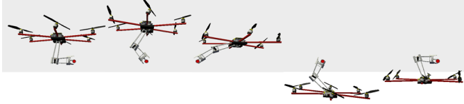
Fig. 3. Time-lapse picture of the aerial manipulator during experiment (I). The end-effector performs a full rotation while the position is constant. Thanks to the optimization the aerial vehicle remains almost horizontal. For clarity: the single time instances are presented next to each other, while in reality, the small red dot in all pictures overlaps.
